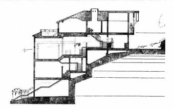
To climb a steep hill, a building becomes a staircase—the retaining walls are its risers and the floors its landings. The Santi residence, designed by Max Jacobson and Murray Silverstein, has eight major landings as it climbs from the dug-in garage to the bedrooms on the highest level.
